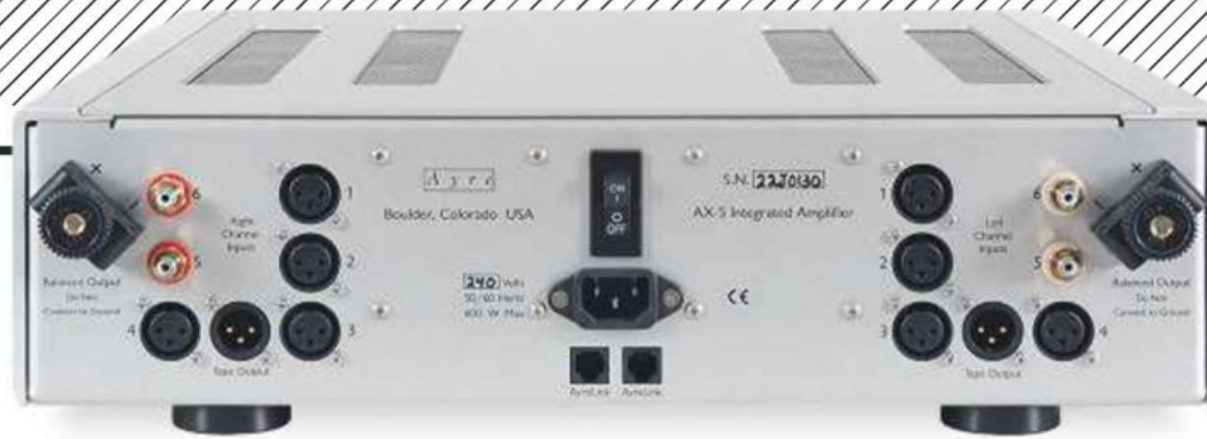
ABOVE: Cardas speaker terminals are joined by four balanced and two single-ended line inputs, plus tape out XLRs. The RJ-11 sockets provide 'AyreLink' system comms
