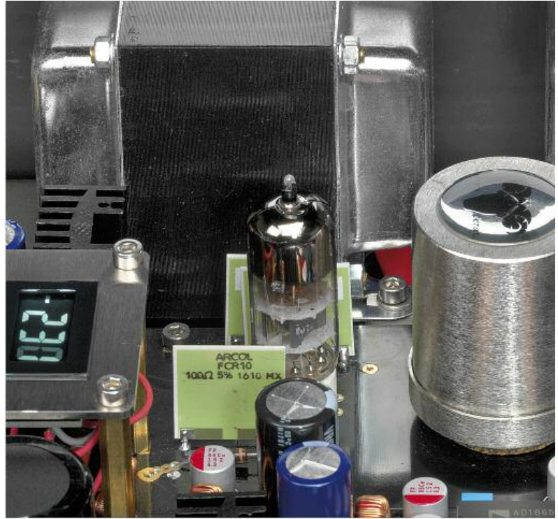
Thick E/I lamination transformers power the tube output stage with channel separation, while specially shielded step-up transformers ensure a low output impedance of 100 ohms
